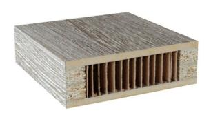
PANOLITE ELEMENT is a component made to customer specifications. It is composed of PANOLITE lightweight panel and of frame elements placed inside the panel according to customer's needs. It is available with the same variety of surface panels and offered in the same choice of finishes as PANOLITE panels. It can be specified unfinished, or factory finished and edgebanded.
