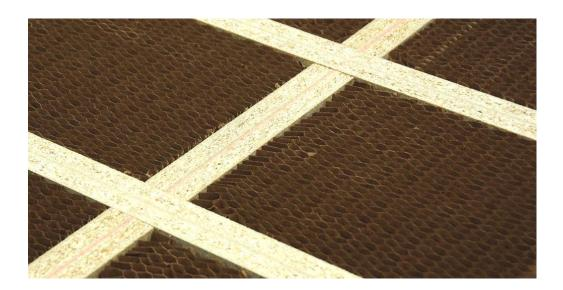
PANOLITE lightweight panels have significant weight advantage over traditional solid or wood panels.
