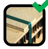
PROTECT CORNERS FROM STRAPPING DAMAGE
