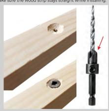
Insert the baffle over the wood strip and secure on both sides using glue with nails or screws\*. Always pre-drill if using screws.
